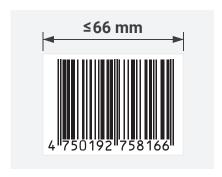
**3.5** If there are requirements for the barcode reading class, both the left and right Quiet Zones must be increased by at least **2 mm**:
